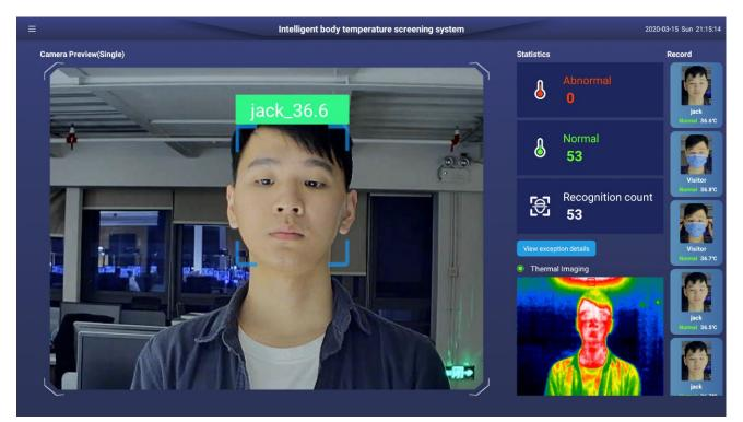
Face recognition and temperature measurement (in mask mode)
